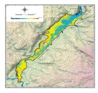
The Sulejów Reservoir is particularly susceptible to eutrophication, caused mostly by long water retention (40 days), low average depth, inflow of waste waters from the direct catchment area and the supply rivers: Pilica and Luciaçãa. The eutrophic character of the waters is caused by excessive load of biogenic substances, especially phosphorus, fed
