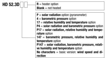
Analog outputs for wind speed and direction: 4...20mA standard; to be requested: 0...1V, 0...5V or 0...10V (0...10V option requires power 15...30Vdc).
